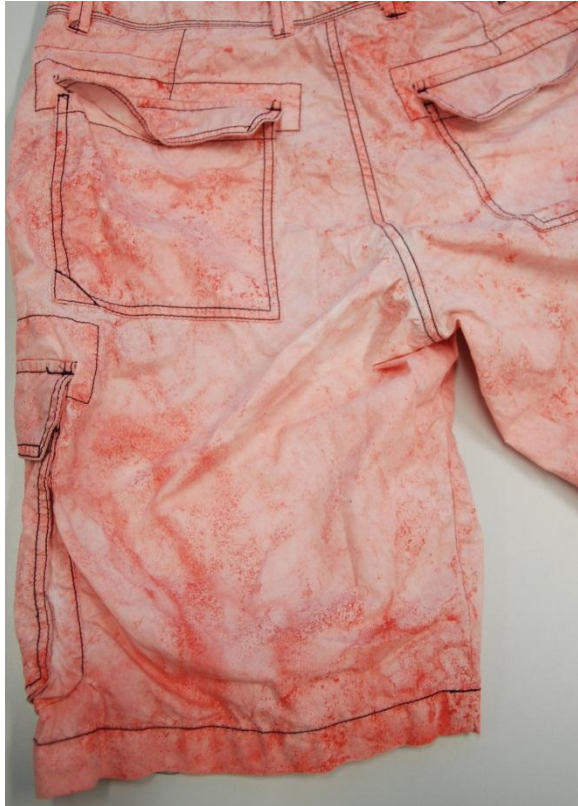
Foam-Dye Dyeing with reactive dyes
