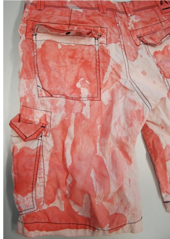
Paint-Dye Dyeing with reactive dyes
