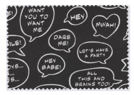
Printed fabric 20 % PERICOAT VA 110 3 % PERICOAT CROSSLINKER MV 6.5 % black pigment
