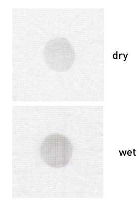
Fastness to rubbing according to DIN EN ISO 105-x-12
